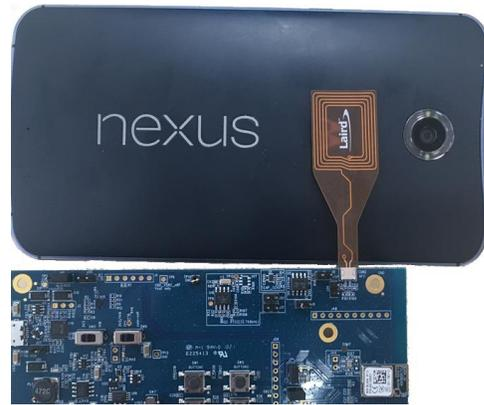
Figure 13: BL654 NFC antenna held flush against android device
