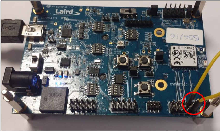
Figure 2: BT900 in VSP mode and jumper attached (front) Pins that the cable is attached: Ground and Pin 19
