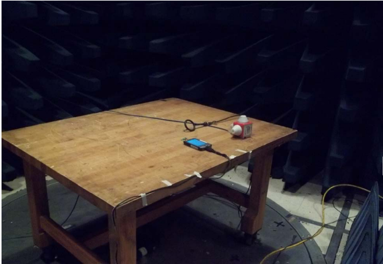
Test Configuration Photograph #2 (Radiated Immunity in Chamber #6, EN 61000-4-3 - EUT in Rx mode)
