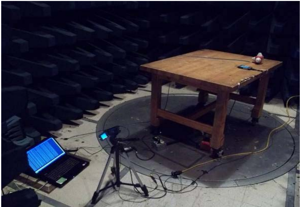
Test Configuration Photograph #1 (Radiated Immunity in Chamber #6, EN 61000-4-3 - EUT in Tx mode)
