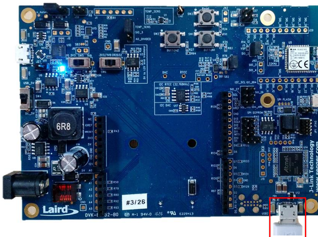
Figure 20: Connecting BL652 to PC through USB2 port
