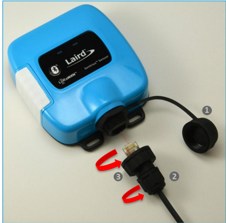
Figure 2: Installing the external temperature sensor
